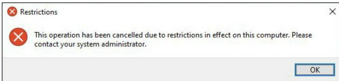
FIGURE 14-6 GPO prohibiting Control Panel access
