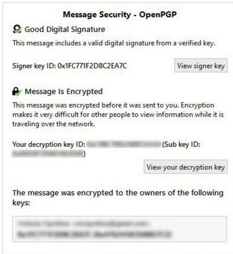
FIGURE 6-6 Good Valid Digital Signature, Message is Encrypted
